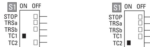
For CAN2, set DIP switch TC2 to the ON position.
