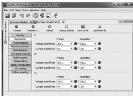
Fig. Display for configuring the current and voltage transformers in the GridVis software.
