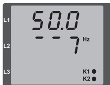
Fig. Display of the mains frequency (50.0) and the rotation field direction
