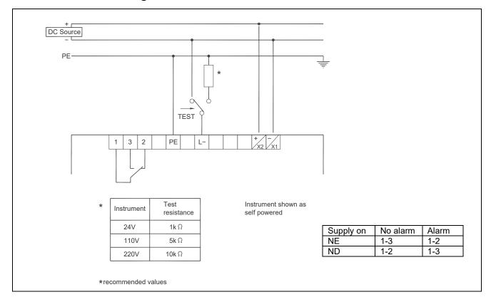
The auxiliary supply should be protected by means of a 2 A fuse.
