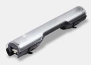
Technical description:LED light-600 lumens, AC/DC supply version, nominal voltage 230<br/>V, operating from 9.6 to 52.8 V (AC) and from 88 to 264 V (DC),<br/>rated power 6 VA, Switching via 0N/0FF switch, Connections: Push-in<br/>terminals for the connection to a single unit, ambient temperature<br/>from -30 to +55 °C
