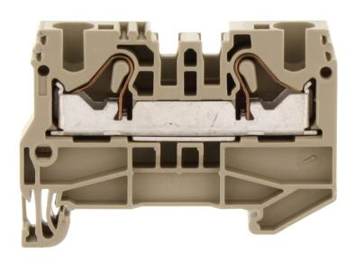
Feed-through installation terminal, Push-in connection, Mounting type: Mounting rail TS 35/7.5, Rated cross-section: 10 mm², Width: 8.1 mm, Colour: Beige
