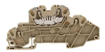
Three-wire installation terminal, Push-in connection, Mounting type: Mounting rail TS 35/7.5, Rated cross-section: 4 mm², Width: 5.1 mm, Colour: Beige
