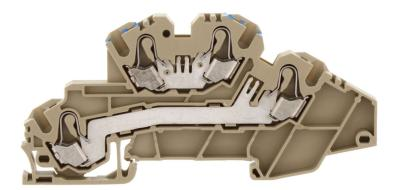
Three-wire installation terminal, Push-in connection, Mounting type: Mounting rail TS 35/7.5, Rated cross-section: 4 mm<sup>2</sup>, Width: 5.1 mm, Colour: Beige
