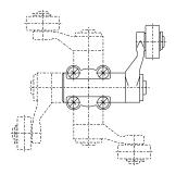
The actuating head can be repositioned by 4 x 90°. Unscrew the four screws of the actuating head (Philips tip profile), reposition the actuating head in the desired position and retighten the four screws (tightening torque 1.5 Nm).
