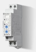
Technical description: Electronic voltage monitoring relays, 1 phase AC line monitoring, 1 pole, 10 A, AC supply version, nominal voltage 230 V, operating from 130 to 280 V, rated power 2.6 VA, Detection values: 2 adjustable detection values, CO (nPDT), Time delay setting: Adjustable switch-off delay, Fault memory option: Fault memory function selectable, ambi-
