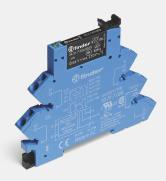
**Technical description:** Relay interface modules, Electromechanical relay, with screwless terminal, 1 pole, CO (nPDT), 6 A, AgNi, DC sensitive coil, 24 V, operating from 19.2 to 28.8 V, rated power 0.3 W, consumption 10.4 mA, holding voltage 14.4 V, must drop-out voltage 1.2 V, option: DC, version: CO
