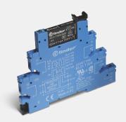
**Technical description:** Relay interface modules, Electromechanical relay, with screw terminal, 1 pole, CO (nPDT), 6 A, AgNi, AC/DC coil, 48 V, operating from 38.4 to 52.8 V (AC)/(DC), rated power 0.3 VA (AC)/(DC), consumption 6.9 mA, holding voltage 28.8 V (AC)/(DC), must drop-out voltage 4.8 V (AC) and 2.4 V (DC), option: AC or AC/DC, ambient temperature from
