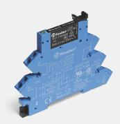
**Technical description:** Relay interface modules, Electromechanical relay, with screwless terminal, 1 pole, CO (nPDT), 6 A, AgNi, AC/DC coil, 24 V, operating from 19.2 to 26.4 V (AC)/(DC), rated power 0.3 VA (AC) / 0.2 W (DC), consumption 12 mA, holding voltage 14.4 V (AC)/(DC), must drop-out voltage 2.4 V (AC) and 1.2 V (DC), option: AC or AC/DC, version: CO
