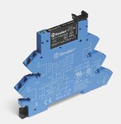
**Technical description:** Relay interface modules, Electromechanical relay, with screwless terminal, 1 pole, CO (nPDT), 6 A, AgNi, AC/DC coil, 12 V, operating from 9.6 to 13.2 V (AC)/(DC), rated power 0.2 VA (AC)/(DC), consumption
