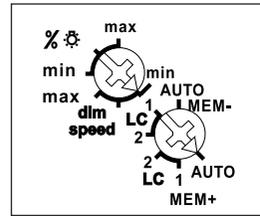
With the **top rotary switch %/dim speed** either the minimum brightness level (completely dimmed down) or the dim speed can be adjusted. The duration of soft-on and soft-off will be changed with the dimming speed.
