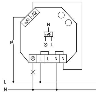
Control voltage, supply voltage and switching voltage 230 V ~ 50/60Hz
