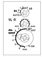
The LED below the rotary switch on the front shows control commands. It starts blinking after 15 seconds if a pushbutton is inhibited. In operation, **the upper rotary switch** determines, whether automatic lamp detection or special comfort positions should operate:
