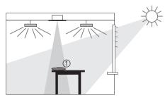
Room correction factor = Brightness value at the ceiling/ brightness value at the working surface
