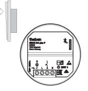
Install in conventional flush-mounted boxes (according to DIN 49073)
