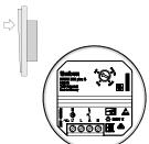
➤ Install in conventional flush-mounted boxes (according to DIN 49073)
