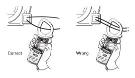
d. Press the trigger to open the transformer jaws and clamp them onto the conductor under test and take the reading on the display
