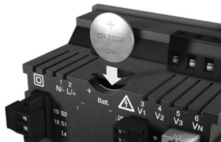
Fig. Battery insertion on the rear
