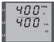
Fig. Programming mode Voltage converter Use button 1 and 2 to change primary and secondary voltage (see page 51).
