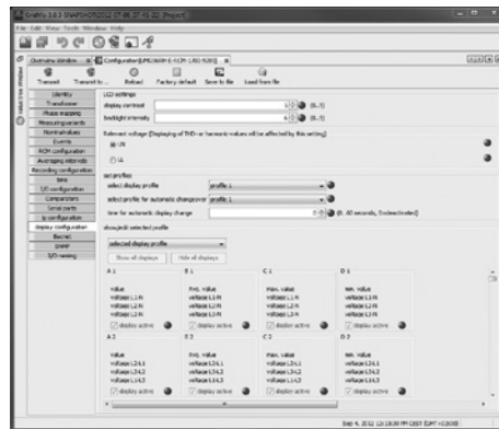
Fig. Profile setting screen in the GridVis software.
