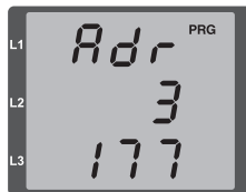
Fig. TCP/IP address Byte 3, value 177
