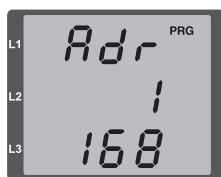
Fig. TCP/IP address, Byte 1 A TCP/IP address consists of 4 bytes with the following structure:
