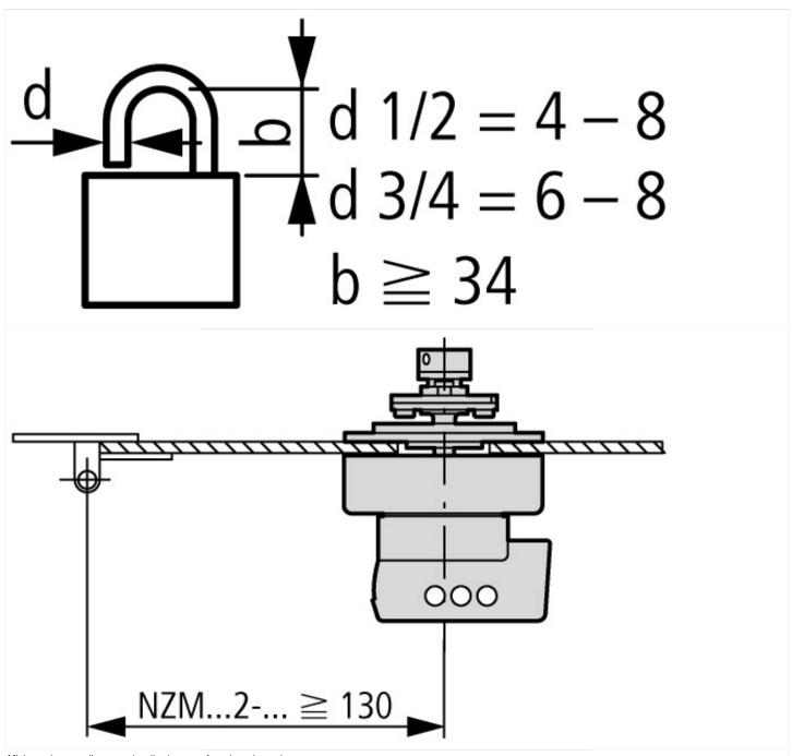
Minimum door coupling rotary handle clearance from door pivot point
