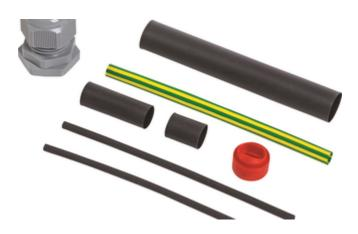
nVent RAYCHEM CE20-01, CE20-03 and CE25-01 are heat shrink polymer kits used to connect and terminate select nVent RAYCHEM self-regulating trace heating cable. Requires wire stripping and a heat gun. Each kit contains connection components for a cable termination and end seal.
